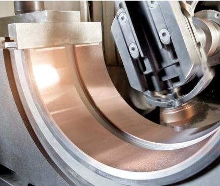
With almost 80 years of experience in crankshaft grinding, our company has also become the specialist in the revision and manufacturing of slide bearings. All common slide bearings are individually manufactured in house.
